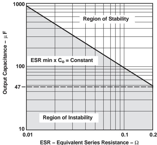
Figure 21. Output Capacitance vs Equivalent Series Resistance
