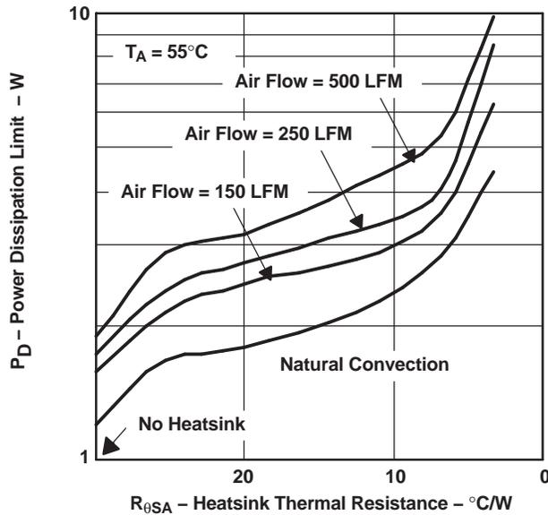
Figure 25. Power Dissipation vs Heatsink Thermal Resistance
