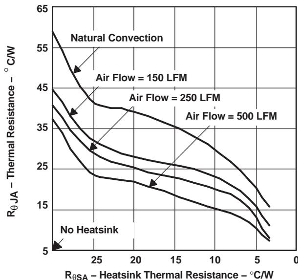
Figure 23. Thermal Resistance vs Heatsink Thermal Resistance
