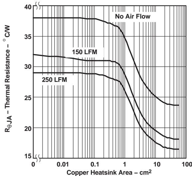
Figure 26. Thermal Resistance vs Copper Heatsink Area
