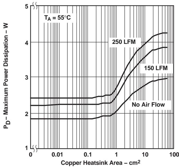
**Figure 28. Maximum Power Dissipation vs Copper Heatsink Area**
