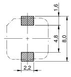
no sensitive traces underneath the component
