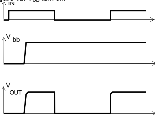
Figure 1a: V_{bb} turn on:
