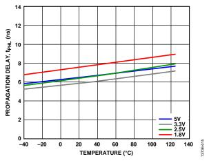
Figure 7. Propagation Delay, t<sub>PHL</sub> vs. Temperature at Various Voltages
