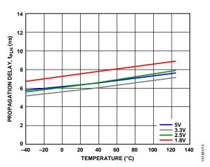
Figure 6. Propagation Delay, t<sub>PLH</sub> vs. Temperature at Various Voltages
