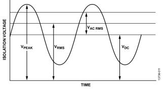
Figure 13. Critical Voltage Example
