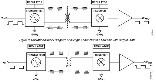
Figure 10. Operational Block Diagram of a Single Channel with a High Fail-Safe Output State
