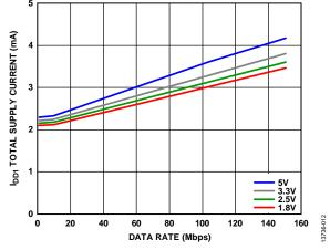
Figure 4. IDD1 Total Supply Current vs. Data Rate at Various Voltages
