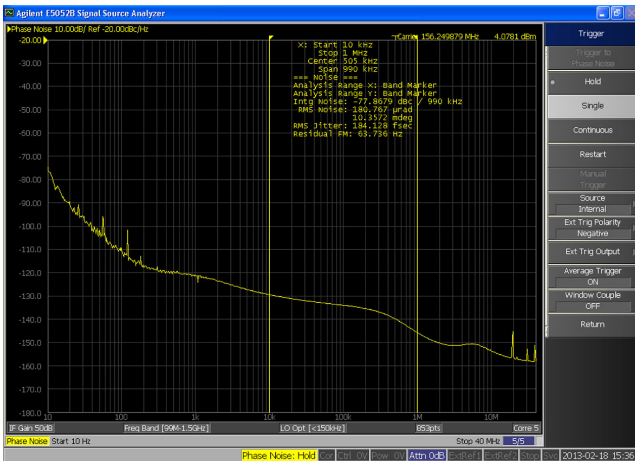
Figure 1. Si535/536 Typical Phase Noise at 156.25 MHz
