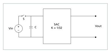
Figure 3 — Sine Amplitude Converter™ with input capacitor
