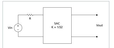
**Figure 2** — *K* = 1/32 Sine Amplitude Converter™ with series input resistor
