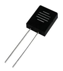
Telaire HS12SP is a bulk-resistance type of Relative Humidity (RH) Sensor providing a variable impedance value in response to the adsorbed water within the sensor's proprietary thin-film polymer. Applied to an interdigitated electrode, the polymer's chemical functional groups disassociate into ionic groups in the presence of water, increasing the sensor's electrical conductivity. Excited by a low voltage alternating current, the sensor's resulting impedance is measured via supporting circuitry.
