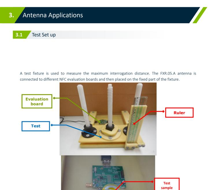
The test sample is placed on a thin sheet of plastic connected to the movable part of the fixture. Then the distance is carefully adjusted until the reader can no longer read the sample, thus the maximum interrogation distance is displayed in the ruler.
