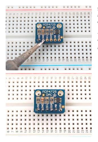
Solder each pin using a soldering iron and solder, to make solid connection on each pin.
