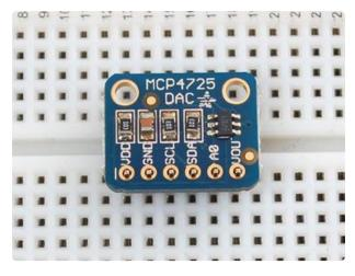
Place the breakout board on top so the short ends of the header stick up through the pads
