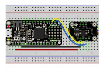
Note: This breakout includes pullup resistors on the I2C lines, no external pullups are required.
