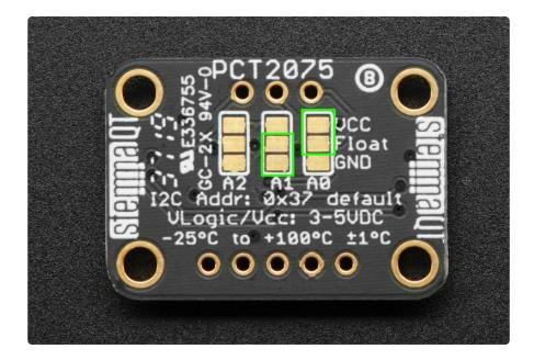
All you need to do is bridge the "Float" pad to either the VCC or GND pad for one or more of the address pins. In the picture above if you bridged the solder pads that are circled, you would pull A0 high to VCC and A1 low to GND. Referring to the table above this would set the address of the breakout to 0x72
