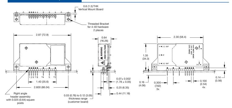
This FS-VM adaptor board provides a convenient way to mount any FS Series high voltage power supply DC to high voltage DC converter on its side, minimizing the X-Y footprint to conserve board real estate. Please note when ordering, the FS Series unit is not included and must be ordered separately.
