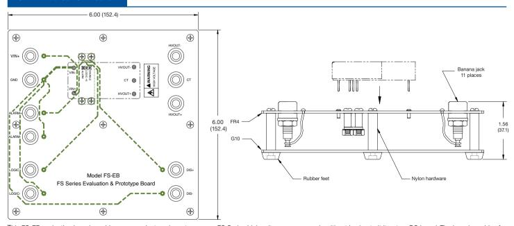
This FS-EB evaluation board provides a convenient package to use any FS Series high voltage power supply without having to it it onto a PC board. The board provides for easy prototyping and evaluation. Please note when ordering, the FS Series unit is not included and must be ordered separately.
