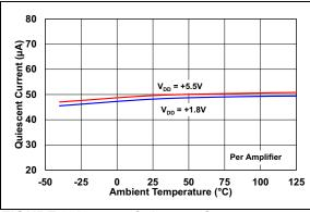
**FIGURE 2-12:** Quiescent Current vs. Ambient Temperature.
