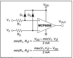
FIGURE 4-3: Protecting the Analog Inputs.
