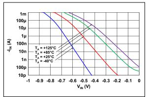
**FIGURE 2-11:** Measured Input Current vs. Input Voltage (below V<sub>SS</sub>).
