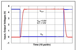
**FIGURE 2-36:** Large Signal Inverting Pulse Response.
