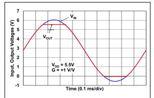
**FIGURE 2-37:** The MCP6006/6R/6U/7/9 Device Shows No Phase Reversal.
