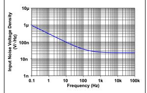
FIGURE 2-28: Input Noise Voltage Density vs. Frequency.
