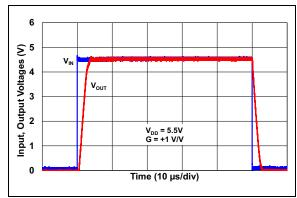
**FIGURE 2-35:** Large Signal Noninverting Pulse Response.
