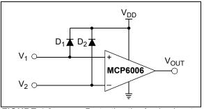
FIGURE 4-2: Protecting the Analog Inputs.
