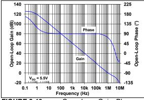
FIGURE 2-19: Open-Loop Gain, Phase vs. Frequency.
