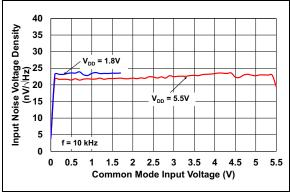
FIGURE 2-27: Input Noise Voltage Density vs. Common-Mode Voltage.
