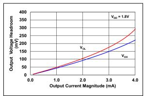
FIGURE 2-16: Output Voltage Headroom vs. Output Current.
