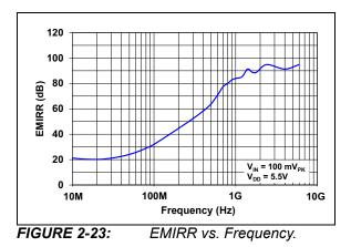
**Note:** Unless otherwise indicated,  $T_A$ = +25°C,  $V_{DD}$  = +1.8V to +5.5V,  $V_{SS}$  = GND,  $V_{CM}$  =  $V_{DD}/4$ ,  $V_{OUT}$  =  $V_{DD}/2$ ,  $V_L$  =  $V_{DD}/2$ ,  $R_L$  = 10 k $\Omega$  to  $V_L$  and  $C_L$  = 30 pF.
