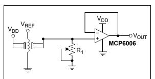
FIGURE 4-10: CO Gas Sensor Circuit.
