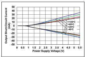
**FIGURE 2-15:** Output Short-Circuit Current vs. Power Supply Voltage.
