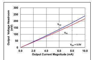
**FIGURE 2-17:** Output Voltage Headroom vs. Output Current.
