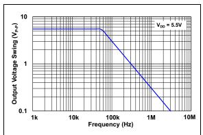
**FIGURE 2-26:** Maximum Output Voltage Swing vs. Frequency.
