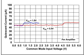
FIGURE 2-14: Quiescent Current vs. Common-Mode Input Voltage.
