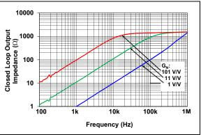
FIGURE 2-22: Closed-Loop Output Impedance vs. Frequency.
