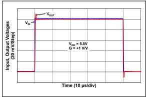
*FIGURE 2-33:* Small Signal Noninverting Pulse Response.
