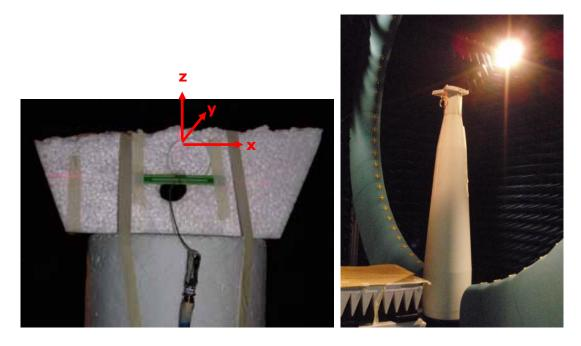
Antenna setup and Satimo SG64 3D-chamber.
