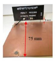
In this position, the antenna is located 2 mm away from the PCB and 3 mm above the PCB
