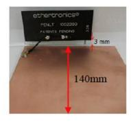
In this position, the antenna is located 3 mm away from the PCB and 3 mm above the PCB
