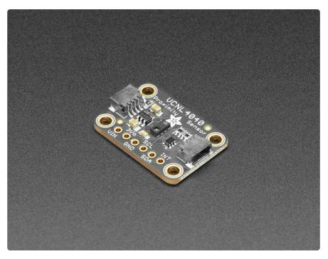
The VCNL4040 is a handy two-in-one sensor, with a proximity sensor that works from 0 to 200mm (about 7.5 inches) and light sensor with range of 0.0125 to 6553 lux.
