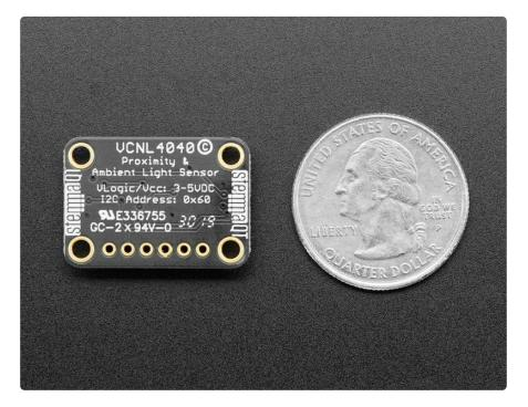
To give you some ability to tune your measurements for your situation, the VCNL4040 lets you adjust the integration time (how long light is being measured) to set the sensitivity of your measurements depending on the lighting conditions. With an integration time of 80ms, since the sensor is only collecting measurements for a short period of time, each measured bit of light represents a larger amount of light. For this reason the maximum range in lux for the 80ms integration time is 6553.5 lux.
