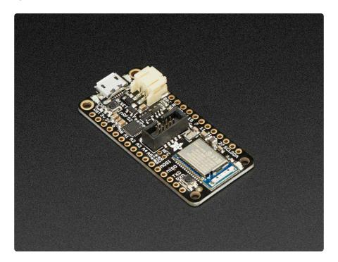
The Adafruit Feather nRF52 Pro is our latest Bluetooth Low Energy board for advanced projects and users who want to use a fully open source Bluetooth Low Energy 5.0 stack. It has a native-bluetooth chip, the nRF52832, as well as built in USB Serial and battery charging! We have other boards in the Feather family, check'em out here. (https://adafru.it/17B)
