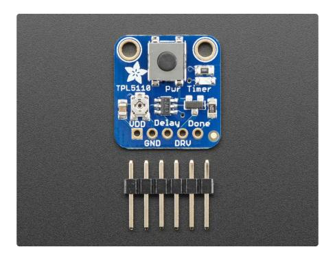
Usage is easy. First, disconnect from power and set your desired delay by adjusting the on-board trim pot: all the way to the left is once-per-100ms an all the way to the right is once-every-2-hours. Then, connect VDD up to your 3-5V power supply and then your project's power-in to the Drive pin. Finally, select a signal pin from your project to the Done pin. In your project's code or design, just make sure that it sets the Done pin high once it is completed with its task. That's it!
