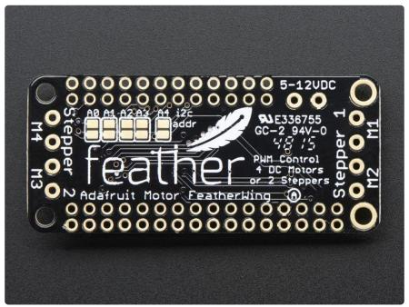
There are two motor sets. The left set is known as Stepper 1 or M1 + M2. The right set is Stepper 2 or M3 + M4
