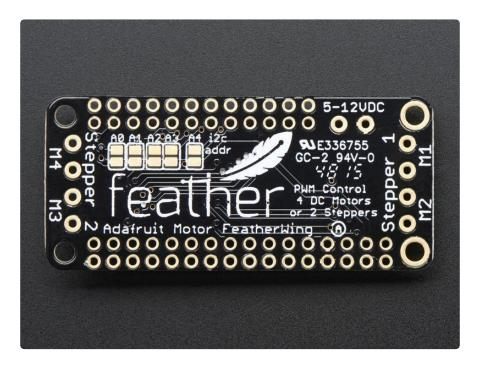
You can stack multiple Motor Wings. Each board in the chain must be assigned a unique address. This is done with the address jumpers on the bottom of the board. The I2C base address for each board is 0x60. The binary address that you program with the address jumpers is added to the base I2C address.
