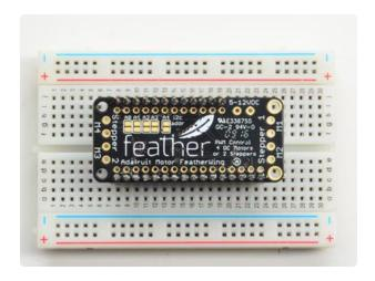
When you are finished, check that your soldered joints are nice and shiny. The rest of the assembly is the same as the non-stacking version.
