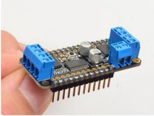
The terminal blocks have interlocking dovetailed grooves on the sides. Line two of them up as shown, and press down to lock them together as a 4-position terminal block. It is a snug fit, so you may have to press hard.
