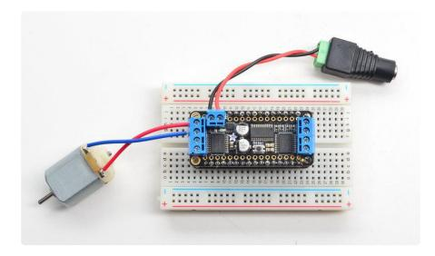
You must also supply 5-12VDC to power the motor. You can power the Wing via a connected DC Barrel Jack as seen above. A battery pack is good for portable use. Note that this will not power the Feather, that's normal - you want to keep separate power supplies and the Feather is best powered by a separate lipoly battery
