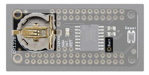
A CR1220 battery holder is on-board for long term RTC timekeeping. A new CR1220 should be able to power the DS3231 for at least 5 years. If you want to use that battery for powering something else (maybe a GPS module or a very low power BLE beacon?) you can connect to the BATT breakout on the very right.
