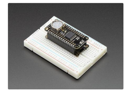
The DS3231 has a default I2C address of 0x68 and cannot be changed
