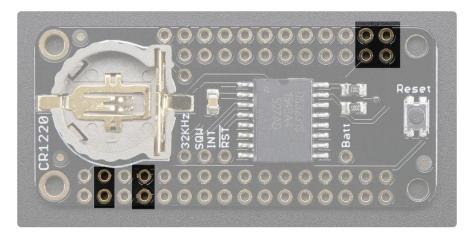
Even though every pin from the Feather is 'doubled up' with an inner header, only 4 of those pins are actually used!
