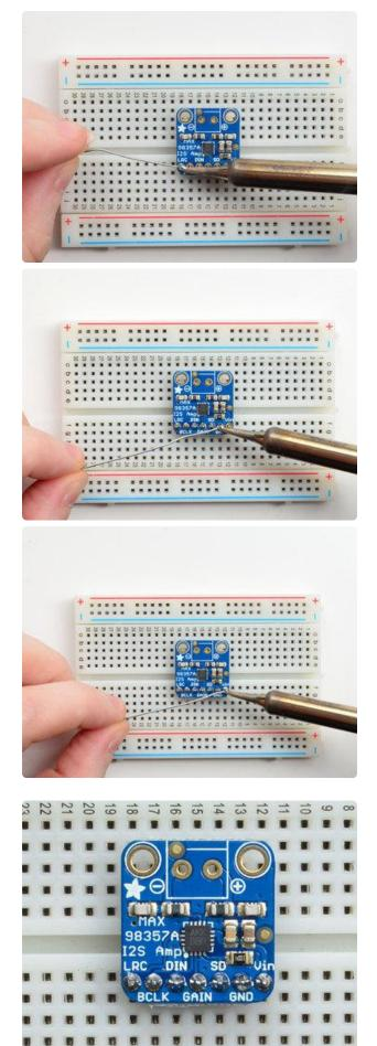
And Solder! Be sure to solder all pins for reliable electrical contact.
