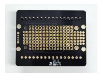
Check the first row once its done, to make sure each pin is shiny and completely soldered
