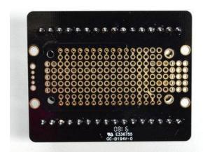
Flip over and solder in one row of the header
