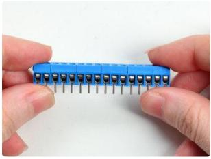
Place the two strips on either side of the breakout PCB with the terminal block holes facing out
