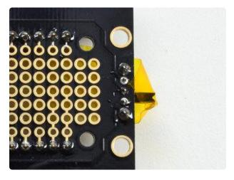
Solder in the two large mechanical points and the three signal pins in the center
