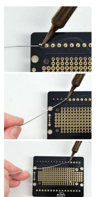
Flip over the board and solder in all of the terminal block pins with plenty of solder
