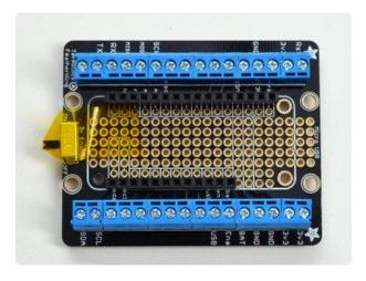
If you'd like to install the slide on/off switch, snap it into place at the end of the PCB and tape it down so it doesn't fall out when soldering
