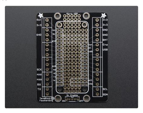
The Terminal Block Featherwing doesn't have any active components. Instead, it just breaks out all the existing connections from a Feather. Note that Feathers use different chipsets so not all pins are labeled on purpose!
