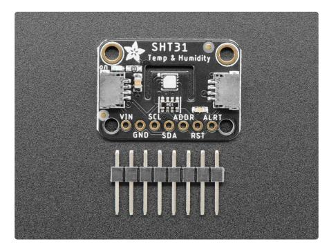
Unlike earlier SHT sensors, this sensor has a true I2C interface, with two address options. It also is 3V or 5V compliant, so you can power and communicate with it using any microcontroller or microcomputer.
