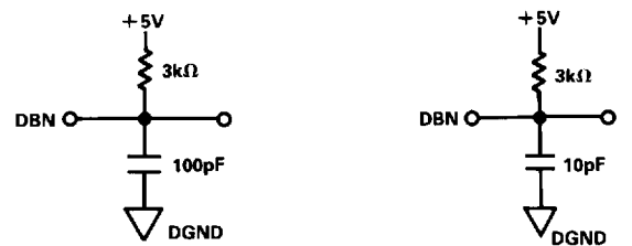
Figure 5. Load Circuit for \overline{INT} Propagation Delays
