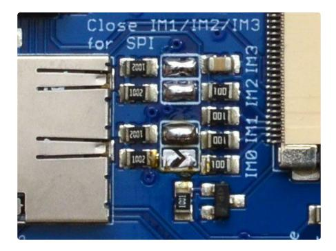
With your soldering iron, melt solder to close the three jumpers indicated IM1 IM2 and IM3 (do not solder closed IM0!)
