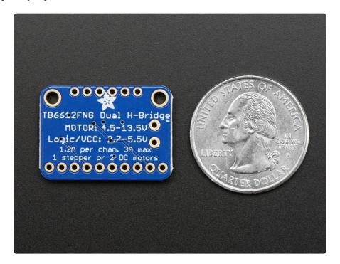
There's two digital inputs per H-bridge (one for each half of the bridge) as well as a PWM input per driver so you can control motor speed. Runs at 2.7V-5V logic. The motor voltage is separate from the logic voltage. Good for motor voltages from 4.5V up to 13.5V! This wont work well for 3V motors.
