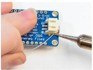
Place the JST and solder that pad onto the connector to tack it in place
