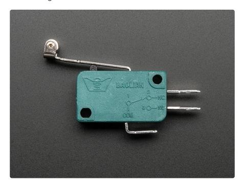
In this case, we connect the COM (common) pin to ground, then the normally-closed to pin #10 and the normally open to pin #0
