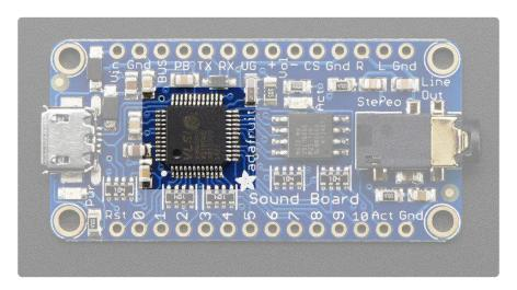
This big chip is the audio decoding engine. It has OGG and WAV decoding capability and can listen to the trigger pins to know when to play each file. It has great audio quality, much better than trying to have a microcontroller generate the audio on its own.
