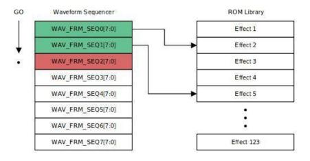
You access the Waveform Sequencer by using the sequence property and providing an index for the slot location. To specify the effect, use the special Effect class provided in the library, giving it the effect number.
