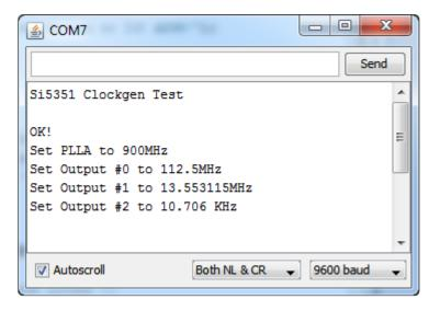
Now you can use your oscilloscope to probe the #0, #1 and #2 outputs
