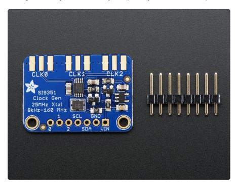
The Si5351 clock generator is an I2C controller clock generator. It uses the onboard precision clock to drive multiple PLL's and clock dividers using I2C instructions. By setting up the PLL and dividers you can create precise and arbitrary frequencies. There are three independent outputs, and each one can have a different frequency.
