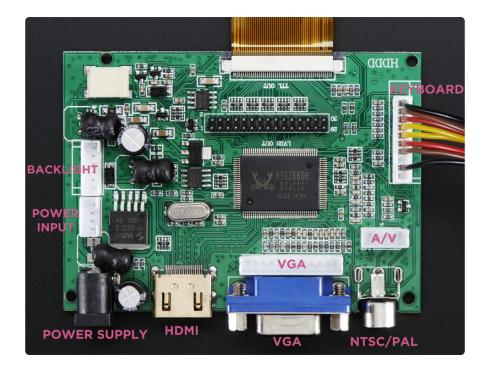
The VGA, Power and A/V inputs, the white JST ports are good alternatives to the main inputs if you don't want bulky cables coming out the sides of your driver board.
