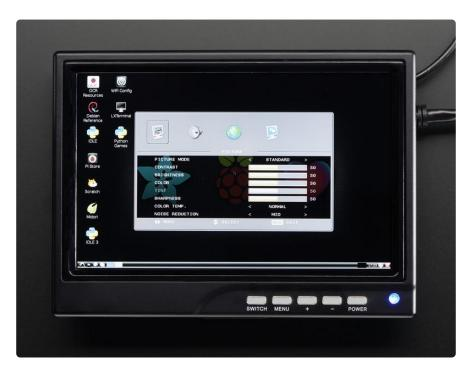
Picture Mode - Standard, Personal, Vivid, Movie Contrast - Adjust the contrast Brightness - Adjust the brightness Color - Adjust the color Tint - Adjust the tint Sharpness - Adjust the sharpness Color Temp - Normal, Cool, Warm Noise Reduction - Mid, Low, Off, High
