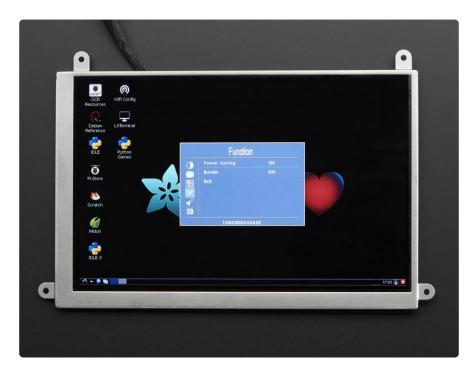
Power Saving - 10s to 60s - how long it takes for the screen to shut off Burnin - On/Off - a function to prevent screen burn-in (https://adafru.it/dTR)
