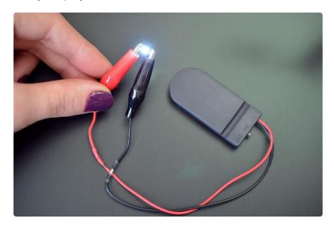
Simply connect 3 to 6VDC to the + pin and ground to the - pin, and the LED on the board will light up. In the photo above we've soldered alligator clips to a 2x2032 coincell battery holder ( $^{\sim}6V$ ). You could also use a single CR2032 sewable coincell holder-- you do not need a microcontroller to drive these sequins, unless you want them to blink or fade.
