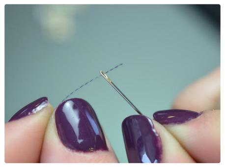
Grab a needle and test it's small enough to pass through the holes in the sequins. Thread up your needle with conductive thread, our 2-ply and 3-ply both are great for this purpose. Check out our conductive thread guide (https://adafru.it/aVx) to learn more about this stainless steel fiber.
