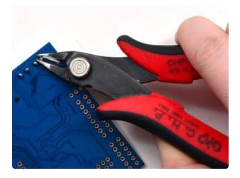
To keep the rightmost speaker pin from bumping into the DC jack you may need to clip it with diagonal cutters
