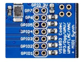
The VS1053 codec chip has 7 'General Purpose Input/Output' pins that you can use to detect button presses and/or light up a small LED. GPIO1 is also used to put it into MIDI mode. By default all these pins are pulled low to ground with 100K resistors. They are 3V logic level so if you want to attach a button, you can connect the two wires between the GPIO pin on the left and the 3V breakout on the right. If you don't want to use these pins just leave them be, they are not required for use!
