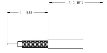
CABLE RECOMMENDED STRIPPING DIM'S. SCALE 3.000
