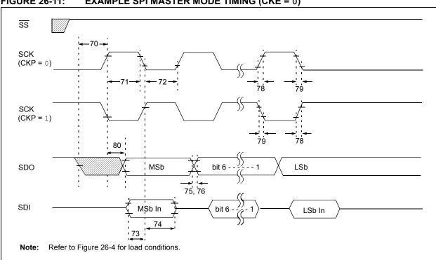
FIGURE 26-11: **EXAMPLE SPI MASTER MODE TIMING (CKE = 0)**
