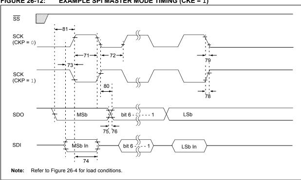
FIGURE 26-12: **EXAMPLE SPI MASTER MODE TIMING (CKE = 1)**
