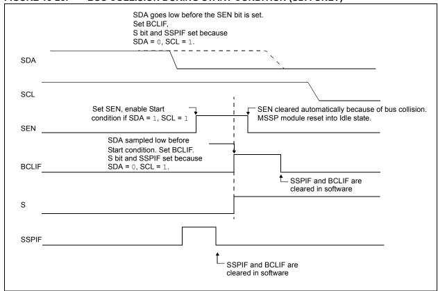
FIGURE 15-27: BUS COLLISION DURING START CONDITION (SCL = 0)
