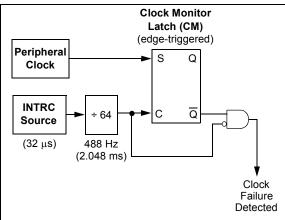
Clock failure is tested for on the falling edge of the sample clock. If a sample clock falling edge occurs while CM is still set, a clock failure has been detected (Figure 23-4). This causes the following:
