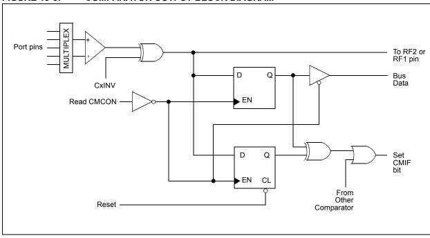
FIGURE 19-3: COMPARATOR OUTPUT BLOCK DIAGRAM
