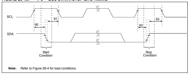
TABLE 26-17: I<sup>2</sup>C™ BUS START/STOP BITS REQUIREMENTS (SLAVE MODE)
