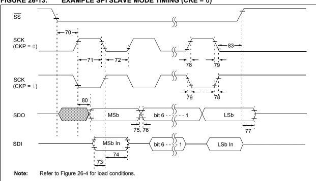
FIGURE 26-13: EXAMPLE SPI SLAVE MODE TIMING (CKE = 0)
