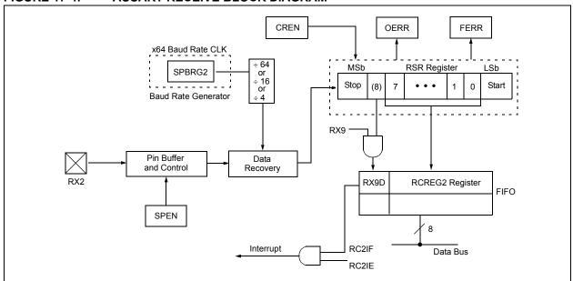
FIGURE 17-5: ASYNCHRONOUS RECEPTION
