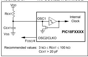
The RCIO Oscillator mode (Figure 2-6) functions like the RC mode, except that the OSC2 pin becomes an additional general purpose I/O pin. The I/O pin becomes bit 6 of PORTA (RA6).
