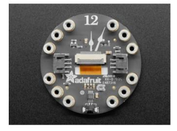
Bolt on this 240x240 pixel color IPS TFT LCD display for bright images, GIFs and animations. You can even fit the LiPoly battery in between the two layers formed by the Gizmo and the Circuit Playground Bluefruit when they are screwed together.
