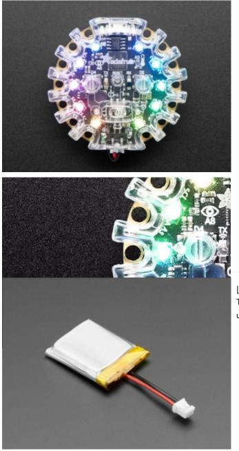
Lithium Polymer Battery The CPB can be powered with this battery for portable use, so it's truly wireless.
