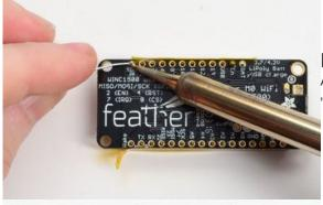
Flip & Tack Solder After flipping over, solder one or two points on each strip, to 'tack' the header in place
