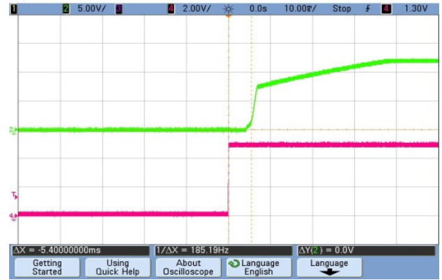
Transient Response (Vin = 12V, Vout = Nom, Iout = 50-75, Cloud = 1µF ceramic||10µF tantalum|| 200µF Ecap; Slew Rate = 1A/µs, Ta = 25°C)
