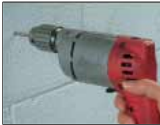
1. Drill hole using correct size bit.
