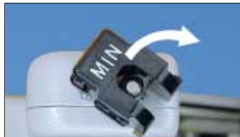
GS2B Tool — Tension Setting Knob
