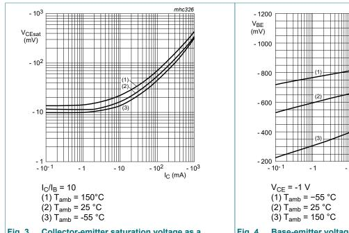
Fig. 3. Collector-emitter saturation voltage as a function of collector current; typical values
