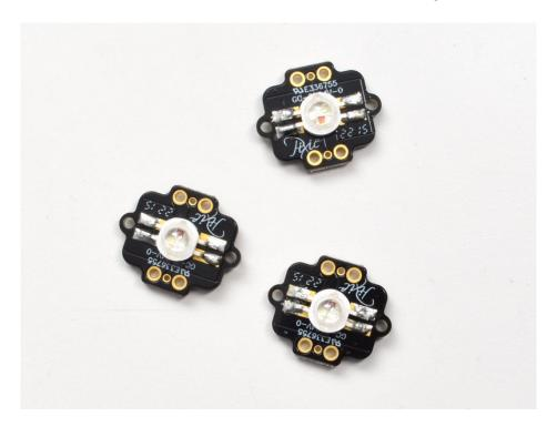
Assembling your Pixies isn't too difficult if you have the right tools and materials. Grab you soldering iron, some thin wire (we like silicone covered 26 AWG) and some thick hefty wire, we used 10AWG stranded.
