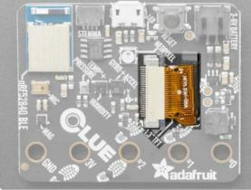
• **1.3**" **240**×**240** Color IPS TFT display - Display high resolution text and graphics. The cable goes through a slot in the board to the back to the display connector.
