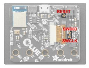
On the bottom of the board are three pads, one near the reset button, and two to the right of the display cable. The pad near the reset button is reset. Of the two pads near the display cable, the top is SWDIO and on the bottom is SWCLK. On the off chance you want to reprogram your CLUE or debug it using a debug/programmer, you will need to solder/connect to these pads.
