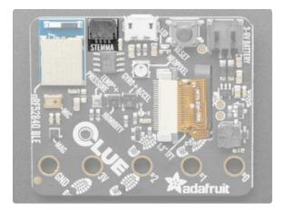
Qwiic / STEMMA QT connector - Use to add more sensors, motor controllers, or displays over I2C. You can plug in GROVE I2C sensors by using an adapter cable (https://adafru.it/IDk).
