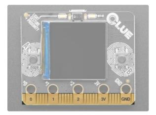
Micro:Bit compatible edge connector - This is the Micro:Bit compatible edge connector, used to break out all of the other features of this microcontroller. Compatible with other Micro:Bit-compatible hardware. While the CLUE is the same outline and we did our best to make the edge-connector pins match up, code may not be immediately compatible without adjustment, especially since only Arduino and CircuitPython are supported at this time.
