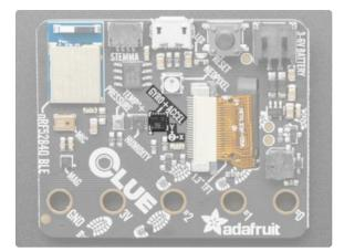
• Gyro + Accel: LSM6DS33 - This sensor is a 6-DoF IMU accelerometer + gyroscope. The 3-axis accelerometer, can tell you which direction is down towards the Earth (by measuring gravity) or how fast the CLUE is accelerating in 3D space. The 3-axis gyroscope that can measure spin and twist. Pair with a triple-axis magnetometer to create a 9-DoF inertial measurement unit that can detect its orientation in real-space thanks to Earth's stable magnetic field. Sensor is I2C on standard pins.
