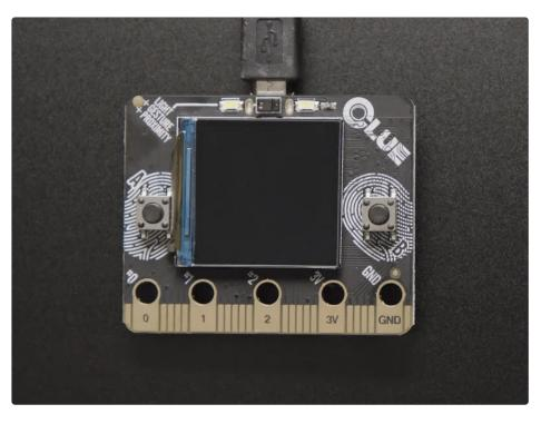
Do you feel like you just don't have a CLUE? Well, we can help with that - get a CLUE here at Adafruit by picking up this sensor-packed development board. We wanted to build some projects that have a small screen and a lot of sensors. To make it compatible with existing projects, we made it the <u>same shape and</u> <u>size as the BBC micro:bit (https://adafru.it/IHB)</u> and with the same edge-connector on the bottom with 5 big pads so it will fit into your existing robot kit or 'bit add-on.
