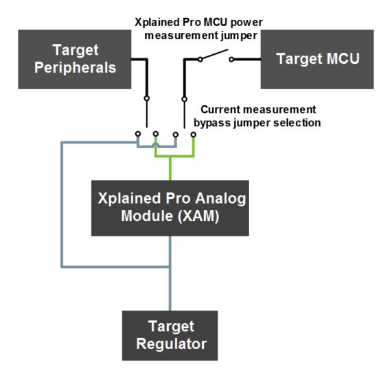
On the SAM R34 Xplained Pro Evaluation Kit, the XAM can be used in four configurations:
