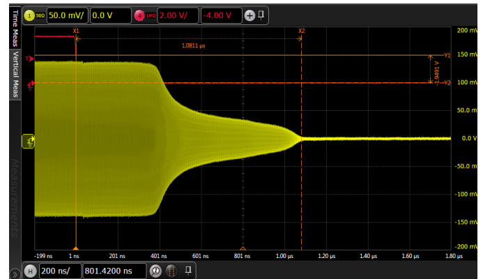
Figure 15. Switching Time [Insertion Loss to Isolation State]
