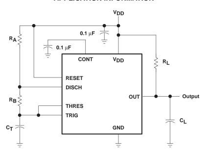
**Figure 1. Circuit for Astable Operation**
