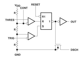
RESET can override TRIG and THRES. TRIG can override THRES.
