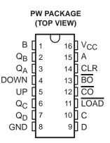
The outputs of the four flip-flops are triggered on a low-to-high-level transition of either count (clock) input (UP or DOWN). The direction of counting is determined by which count input is pulsed while the other count input is high.
