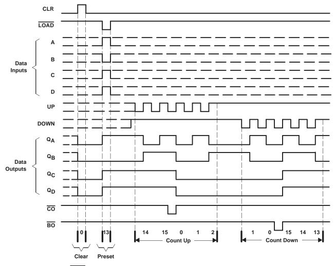
NOTES: A. CLR overrides LOAD, data, and count inputs. B. When counting up, count-down input must be high; when counting down, count-up input must be high.
