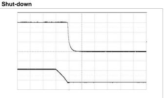
Shut-down enabled by disconnecting V<sub>I</sub> at:  $T_{P1} = +25^{\circ}C$ , V<sub>I</sub> = 53 V,  $I_{O} = 8.5$  A resistive load.
