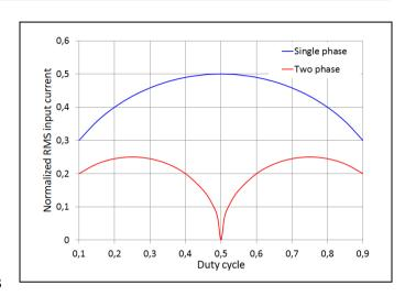
The input ripple RMS current in a two-phase buck converter can be estimated to
