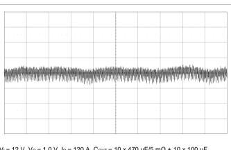
$V_I$  = 12 V,  $V_O$  = 1.0 V,  $I_O$  = 120 A,  $C_{OUT}$  = 10 x 470  $\mu F/5$   $m\Omega$  + 10 x 100  $\mu F,$  5 mV/div, 50  $\mu s/div$
