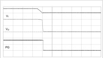
Output disabled by removing V<sub>I</sub>.  $V_I$  = 12 V,  $I_O$  = max  $I_O$ . Scale from top: 10, 0.5, 2 V/div, 1 ms/div.
