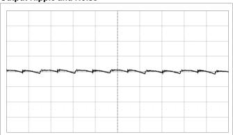
Fundamental output voltage ripple at V $_I$  = 12 V, I $_0$  = max I $_0$ , C $_{OUT}$  = 10 x 470  $\mu$ F/5 m $\Omega$  + 10 x 100  $\mu$ F. Scale: 10 mV/div, 2  $\mu$ s/div, 20 MHz bandwidth. See section Output Ripple and Noise.
