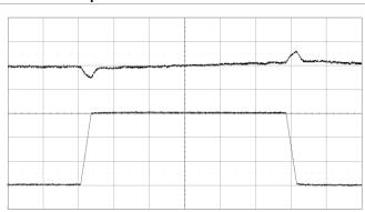
Output voltage response to load current step change (30–90–30 A) at V<sub>I</sub> = 12 V, C<sub>OUT</sub> = 10 x 470  $\mu\text{F/5}$  m $\Omega$  + 10 x 100  $\mu\text{F}$ , di/dt = 2 A/ $\mu\text{s}$ , ASCR Gain = 300 and ASCR Residual = 90. Scale from top: 50 mV/div, 20 A/div, 100  $\mu\text{s}$ /div.
