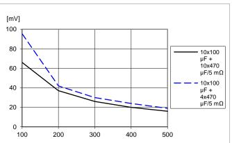
Load transient peak voltage deviation vs. ASCR gain and external capacitance.
