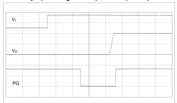
Output enabled by applying  $V_1$ .  $V_1$  = 12 V,  $I_0$  = max  $I_0$ . TON\_DELAY = TON\_RISE = 5 ms, POWER\_GOOD\_DELAY = 2 ms. USER\_CONFIG = 0x1480 (default). PG pulled up to external voltage. Note: PG being high before Vin applied can be avoided by pulling up PG to Vout. Scale from top: 10, 0.5, 2 V/div, 20 ms/div.
