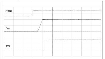
Output enabled by CTRL pin.  $V_1$ = 12 V,  $I_0$ = max  $I_0$ . TON\_DELAY = TON\_RISE = 5 ms, POWER\_GOOD\_DELAY = 2 ms. Scale from top: 5, 0.5, 2 V/div, 10 ms/div.
