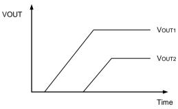
Illustration of output voltage sequencing.
