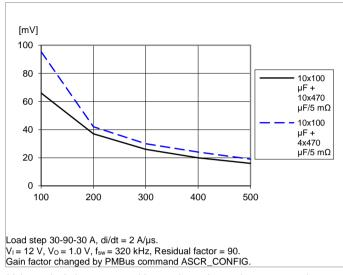
Voltage deviation vs. control loop gain setting and output capacitance.
