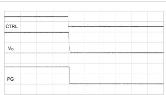
Output disabled by CTRL pin.  $V_1 = 12 \text{ V}$ ,  $I_0 = \text{max } I_0$ . Scale from top: 5, 0.5, 2 V/div, 1 ms/div.
