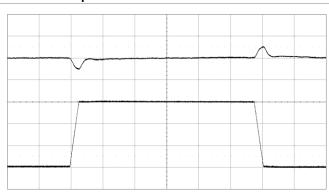
Output voltage response to load current step change (30–90–30 A) at V $_{I}$  = 12 V, C $_{OUT}$  = 10 x 470  $\mu F/5$  m $\Omega$  + 10 x 100  $\mu F,$  di/dt = 2 A/ $\mu s,$  ASCR Gain = 300 and ASCR Residual = 90. Scale from top: 50 mV/div, 20 A/div, 100  $\mu s$ /div. Note: Sense pins are connected to load.
