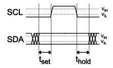
Setup and hold times timing diagram.
