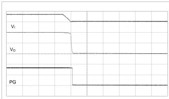
Output disabled by removing  $V_I$ .  $V_I = 12 \ V$ ,  $I_O = max \ I_O$ . Scale from top: 10, 0.5, 2 V/div, 1 ms/div.
