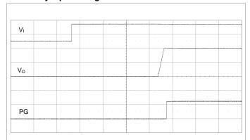
Output enabled by applying V<sub>1</sub>. V<sub>1</sub> = 12 V, I<sub>0</sub> = max I<sub>0</sub>. TON\_DELAY = TON\_RISE = 5 ms, POWER\_GOOD\_DELAY = 2 ms. USER\_CONFIG = 0x1484 (PG push-pull). Scale from top: 10, 0.5, 2 V/div, 20 ms/div.
