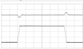
Output voltage response to load current step change (30–90–30 A) at V<sub>I</sub> = 12 V, C<sub>OUT</sub> = 10 x 470  $\mu F/5$  m $\Omega$  + 10 x 100  $\mu F,$  di/dt = 2 A/ $\mu s$ , ASCR Gain = 300 and ASCR Residual = 90. Scale from top: 50 mV/div, 20 A/div, 100  $\mu s$ /div.
