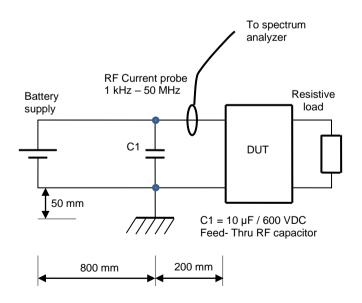
Test set-up conducted emission, power lead. DUT = Product mounted on a 182 cm² test board with the external capacitances  $C_{\text{IN}}$  = 1000  $\mu$ F/12 m $\Omega$  + 24 x 10  $\mu$ F and  $C_{\text{OUT}}$  = 10 x 470  $\mu$ F/5 m $\Omega$  + 10 x 100  $\mu$ F.
