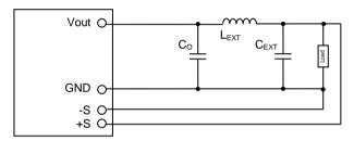
External output filter with inductor (PI filter).
