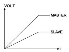
Illustration of ratiometric voltage tracking.
