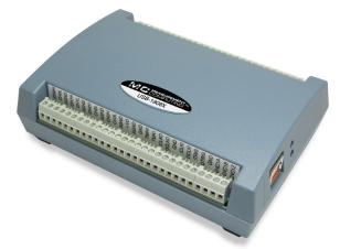
USB-1808 Series devices provide eight simultaneously-sampling analog inputs that are configurable per channel as differential or single-ended, two analog outputs, four digital I/O, two general-purpose counters, two quadrature encoders, and two timer outputs.
