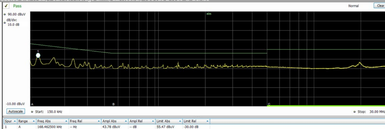
EMI; Conducted CISPR 22; Peak vs. Average Limit; L2/Neutral; 100Vac 24Vdc @ 25Adc
