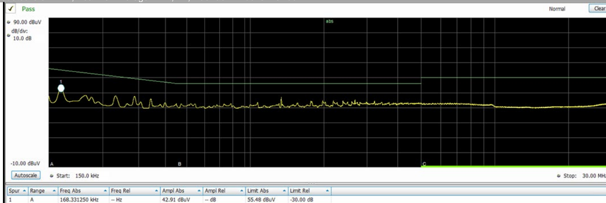
EMI; Conducted CISPR 22; Peak vs. Average Limit; L2/Neutral; 100Vac 24Vdc @ 25Adc
