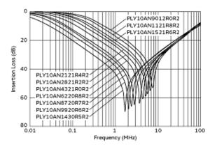
Differential Mode Insertion Loss-Frequency Characteristics
