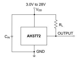
Note: 4. C<sub>IN</sub> is for power stabilization and to strengthen the noise immunity, the recommended capacitance is 10nF ~ 100nF. R<sub>L</sub> is the pull-up resistor.
