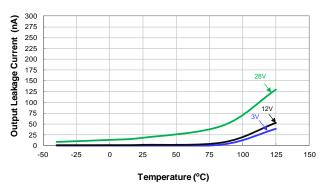
Output Leakage Current vs Temperature
