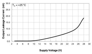
Output Leakage Current vs Supply Voltage
