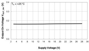
Output On Voltage vs Supply Voltage
