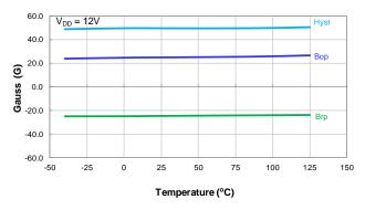
Switch Points BOP and BRP vs Temperature
