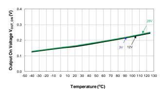
Output On Voltage vs Temperature
