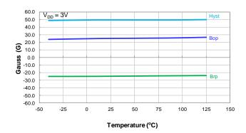
Switch Points BOP and BRP vs Temperature
