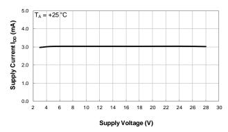
Supply Current vs Supply Voltage
