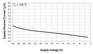
Supply Reverse Current vs Supply Voltage
