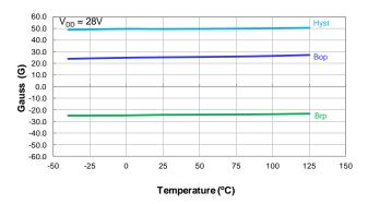
Switch Points B<sub>OP</sub> and B<sub>RP</sub> vs Temperature
